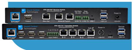
Designed for Cisco codecs, Poly codecs, and 3<sup>rd</sup> party solutions, the RTK-AM1<sup>™</sup> provides simple extension from the codec to the table using a single CAT cable up to 100M. The RTK-AM1 includes an integrated 4x1 video switch with 1 USB-C and 3 HDMI inputs. The USB-C port supports audio, video, data and laptop power for a single cable user experience. The RTK-AM1 can accommodate up to four PoE devices on combined or separated VLANs.
